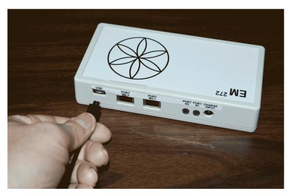
For the EM272, make sure the unit is OFF and plug the Mini-USB cable into the mini-USB jack. The EM272 is OFF if the green LED ring light is not lit.
